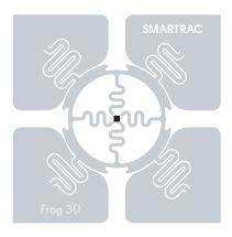
Frog 3D tags and inlays are designed for pallet and case level applications offering high performance in supply chain management applications.
