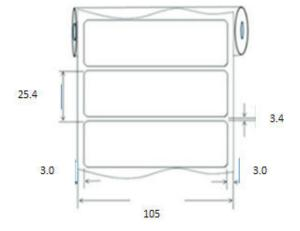
Dimensions stated in mm Supply format = 1000 labels per roll
