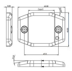
Dimensions stated in mm Attachment hole diameter = 5.2mm
