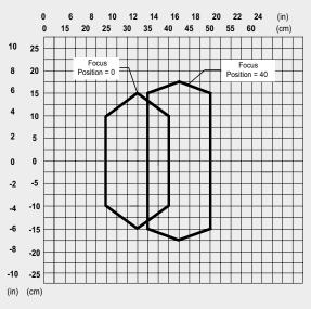
**CONDITIONS**Code = Interleaved 2/5 or Code 39 PCS = 0.90Pitch angle = 0° Skew angle = 10° - 20° Tilt angle = 0
