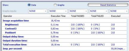
The statistics panel displays all the information about inspection results and execution time. Data can be shown also in a graph.
